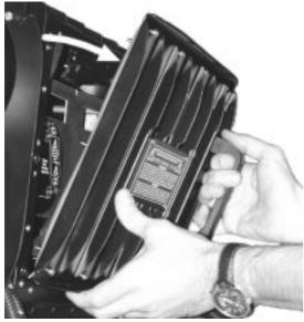
3) Identify the two lamp assemblies, right and left, and, using a Philips head screwdriver, remove the three screws (**C**) which affix the lamp assembly.
