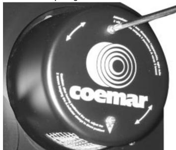
The fans and air inlets must be cleaned regularly to ensure the unit operates correctly. This should be underaken at least every 6 weeks, the period for this periodic cleaning will depend, of course, upon the conditions in which the projector is operating.
