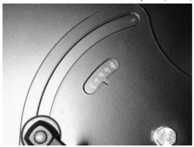
After having set up the position as required, remember to tighten the knobs once again to avoid movement.
